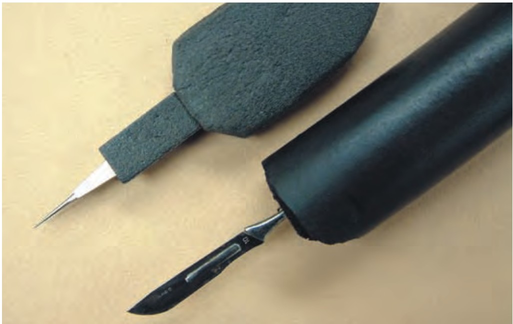
Fig. 5. Insulated tweezers (top) and a scalpel (bottom) used to freeze-fracture specimens in preparation for SEM. Black adhesive rubber foam insulation was cut to size and attached to the tools shown.
